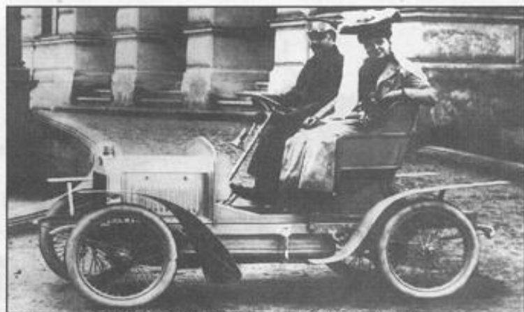
A Type A Laurin & Klement 7hp voiturette of 1906 with v-twin engine.
